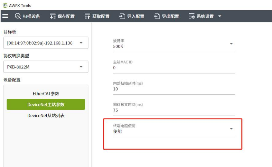
Figure 2.4 Terminal resistance configuration interface
