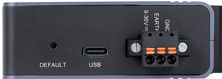
Figure 2.2 Top interface definition diagram
