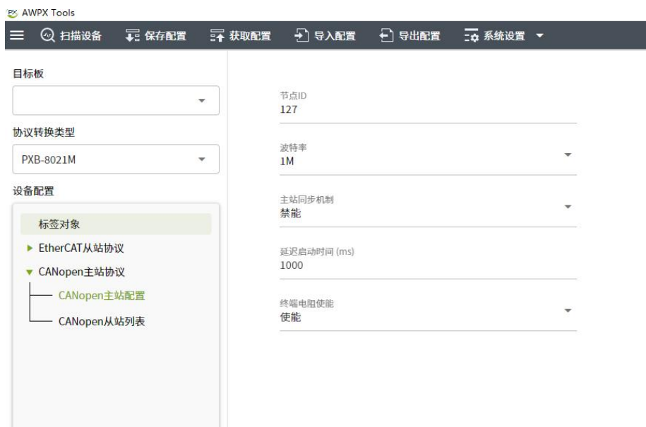
Figure 3.52 CANopen Master Station Parameter Configuration Interface
